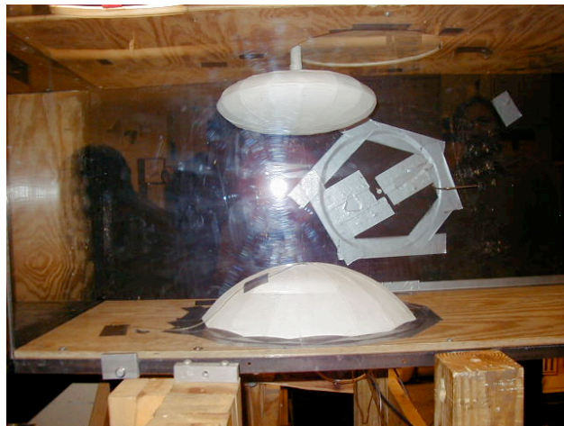
Figure 3. Experimental Setup for Pressure Measurements in the Low Speed Wind Tunnel.
